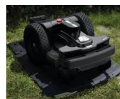
Station de charge
